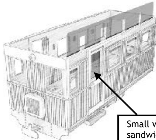
Small window pane, sandwiched between door frame and long window pane.
