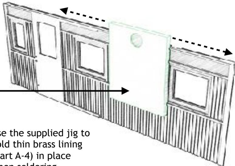
Use the supplied jig to hold thin brass lining (part A-4) in place when soldering.
