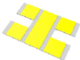
**3** Take the thin-as-paper PCB board and cut it as an 'H'. Make this 2 times (for front and rear light).
