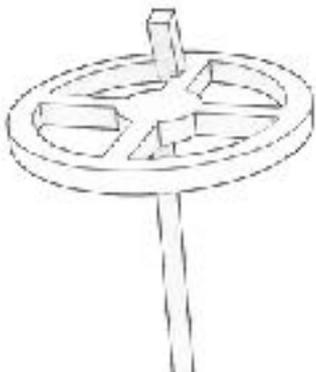
Solder the wheel on a piece of the supplied 0.3 brass wire. It easiest to pre-solder the top of the wire and put flux in the hole. Stick the brass wire in foam to keep it straight up.
