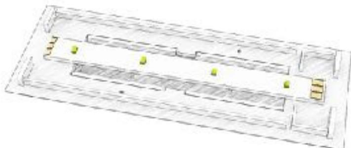
**1** Take the Train-O-Matic LED light strip (B-16) and cut it to size, as shown on the picture. Tape it with double sided tape to the roof, the part where it is cut to the rear of the train.
