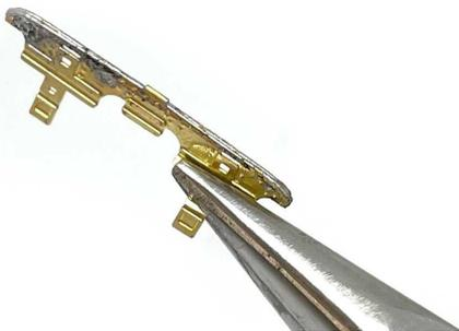
Put solder or super glue on the parts that you've just folded, so all parts fall on top of each other. This includes the "harmonica", which now can be closed completely. Make sure the alignment is correct. Check the back so that the holes are aligned.
