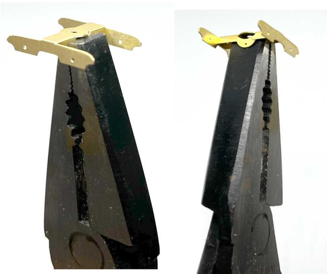
Use pliers to fold the two side wings of the centre part of the frame. You might have to overbend these parts as well, so 95 degrees. This is so the wheels don't touch it.
