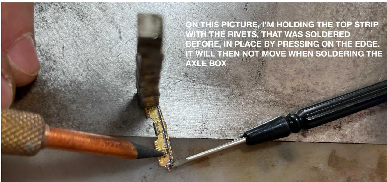
ON THIS PICTURE, I'M HOLDING THE TOP STRIP WITH THE RIVETS, THAT WAS SOLDERED BEFORE, IN PLACE BY PRESSING ON THE EDGE. IT WILL THEN NOT MOVE WHEN SOLDERING THE AXLE BOX
