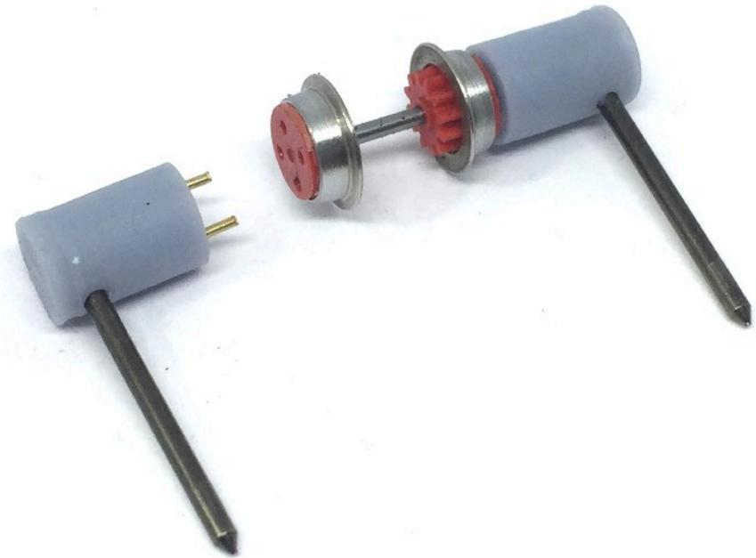
Not all wheels are quartered correctly. With this tool it is easy to align them. Just turn on the handles until the holes on both wheels are in line with each other. The coupling rod on one side should be mounted 90 degrees different from the other side.
